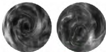
Figure 3 Two snapshots of the flow at Wi = 13 Re = 0.7 . The flow under the black upper plate is visualized by seeding the fluid with light reflecting flakes (1% of the
